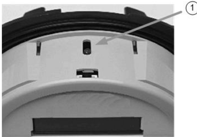
Figure 34: Test LED Location
